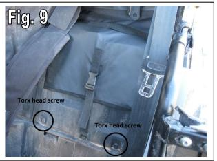
**8.** Start with the top corner straps and evenly tighten each strap. Work your way from top to bottom and tighten all straps. Reinstall your seats. Check your work and be sure everything is tight and secure. You are now ready to ride with your new Tusk Rear Window!
