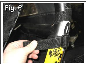
**6.** Next, route the bottom corner straps down around the base of the B-pillar and under the bar that the door hinges on. Thread strap through buckle as seen in figure 7. Leave straps somewhat loose for now.
