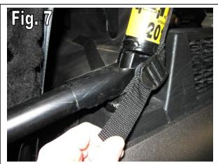
7. Unbuckle the two straps with the plastic hooks attached to them on the bottom of the rear window. Slide the plastic hooks under the back panel/engine cover (see fig. 8). Align the strap with the female buckle on the rear window. Reinsert the male buckle in the female buckle. Leave somewhat loose for now. <u>Tip:</u> It may help to loosen the four Torx head screws that attach the plastic back panel/engine cover (see fig. 9).
